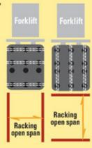
Metal Support Struts - Reduces the pallet's deflection and increase racking load.
